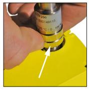
For mounting the sensor must be plugged into the socket and screwed on the sensor by turning the lower knurled screw clockwise. Tighten hand-screwed only. A small clearance between transmitter and sensor has to be accepted due to production conditions.
